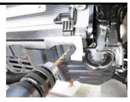
Use Back stop to protect radiators while drilling.
